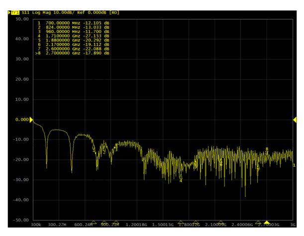
VSWR – Voltage standing wave ratio of LTE antenna [-]
