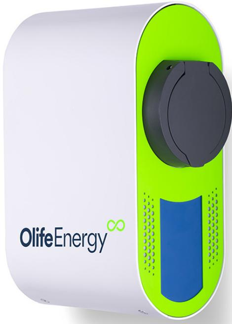
OlifeEnergy WallBox is an all-metal heavy-duty charging station for charging of all electrical vehicles with AC and with a total output of up to 22 kW. It is intended for indoor and outdoor use, with an option of being installed on the wall or a profile anchored in the ground (column). Upon customer's wish, WallBox can be equipped with a socket or a cable (Type 2 as well as Type 1), or with a special coiled cable.
