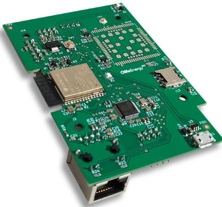
**OlifeEnergy SolarModule** is extension module for all models of OlifeEnergy AC chargers which enables direct communication with selected photovoltaic inverters.
