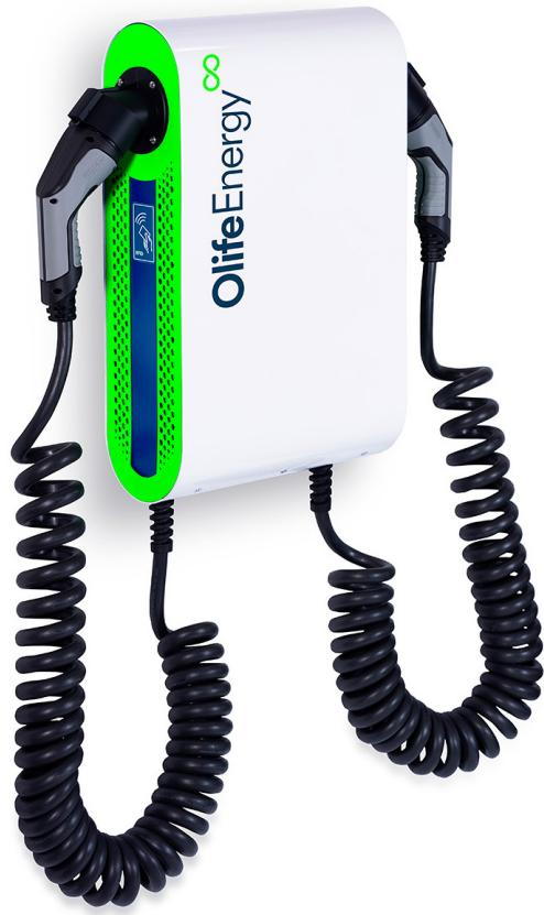
OlifeEnergy DoubleBox is an all-metal heavy-duty charging station for charging of two electrical vehicles with AC and with a total output of up to 44 kW (22 kW each). It is intended for indoor and outdoor use, with an option of being installed on the wall or a profile anchored in the ground (column). Upon customer's wish, DoubleBox can be equipped with a socket or a cable (Type 2 as well as Type 1), or with a special coiled cable.
