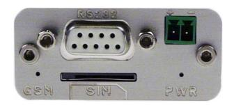
RS232 - Connector for terminal connection via RS232
