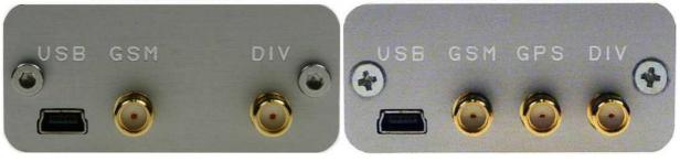
USB – USB connector for connection to computer
