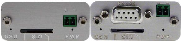
GSM – LED is inactive after the device is switched on; function can be set by command AT^SLED (option cannot be saved)
