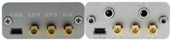
USB – USB connector for connection to computer
