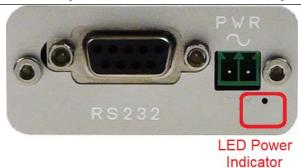
RS232 — Connector for terminal connection via RS232
