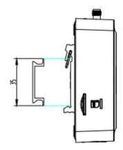
Use 3 pcs of M3 screws to mount the router on the DIN rail, and then hang the DIN rail on the holder. You need to choose a standard holder.
