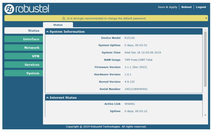
In the home page, the user can save the configuration, restart the router, log out, and so on.
