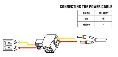
R1510 Router supports reverse polarity protection, but always refers to the figure above to connect the power adapter correctly. There are two cables associated with the power adapter. Following to the color of the head, connect the cable marked red to the positive pole through a terminal block, and connect the yellow one to the negative in the same way.
